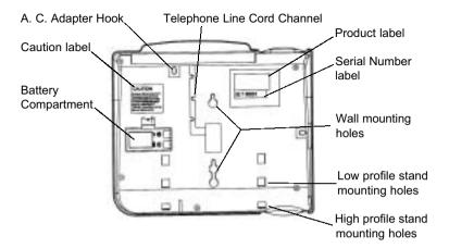
A. C. Adapter Hook: Secures the A. C. Adapter wire, preventing accidental removal.
